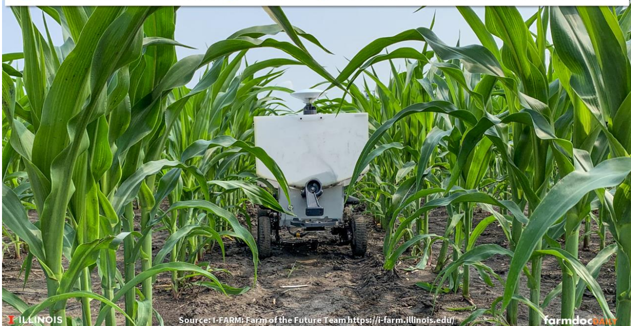
Figure 5. Robot Distributing Cover Crop Seed at I-FARM: Farm of the Future
